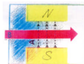
Fig. 3: Effective factors in the magnetic field A: Lines of the magnetic field B: Direction of the fluid
